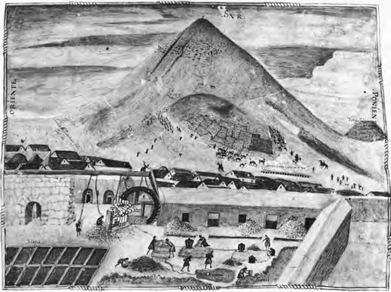
POTOSÍ. Honeycombed with mine shafts, the “mountain of silver” looms over the city of Potosí in modern Bolivia—called Upper Peru at the time of this 1584 painting. In the foreground, silver ore is being crushed by water-powered machinery and mixed with mercury to extract the precious metal. The Granger Collection, New York.
